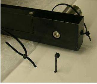
Figure 4.12 *Example of how to fasten tie wraps*
