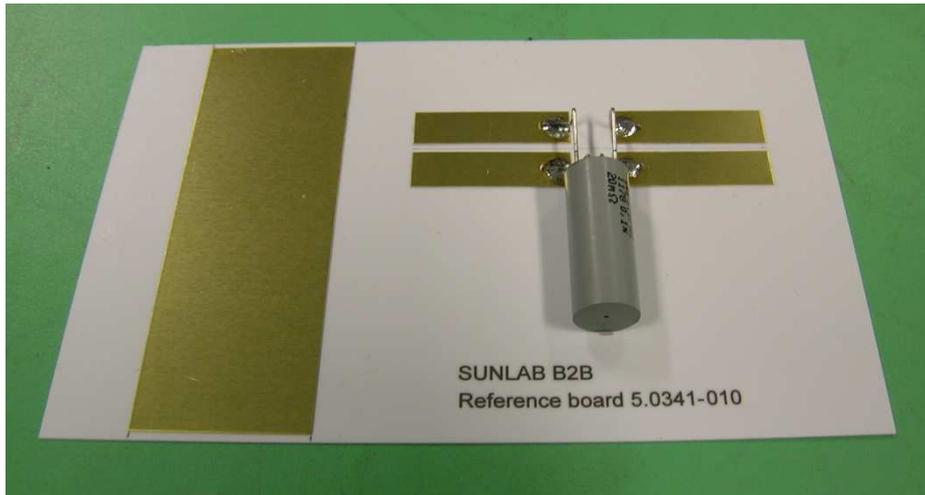
Figure 4.10 *B2B test board for checking operation*
