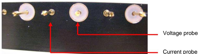
Figure 4.9 *Voltage probe and current probe close-up*
