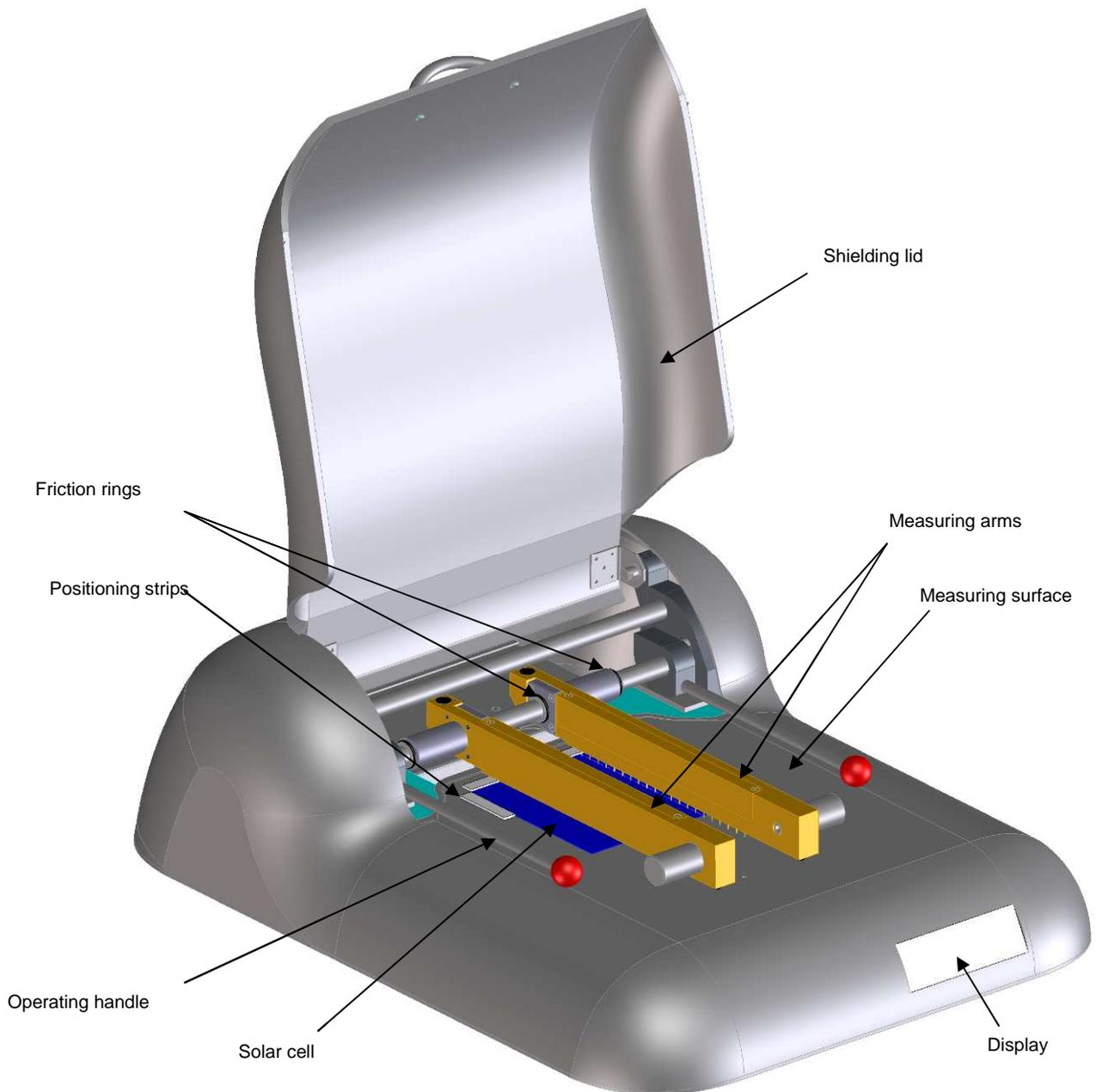
Figure 2.1 *SunLab B2B definitions of system components*
