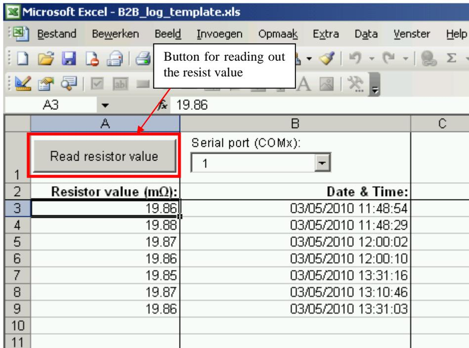
Figure A.1 Excel log sheet 'Read resistor value'
