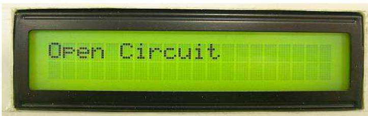
Figure 4.5 *Display 'open circuit'*
