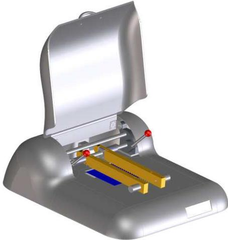
Figure 3.2 *Adjustment of the width of the measuring arms*
