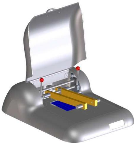
Figure 3.1 *Replace solar cell*
