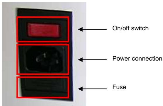
Figure 4.1 *On/off switch at the rear of the SunLab B2B*
