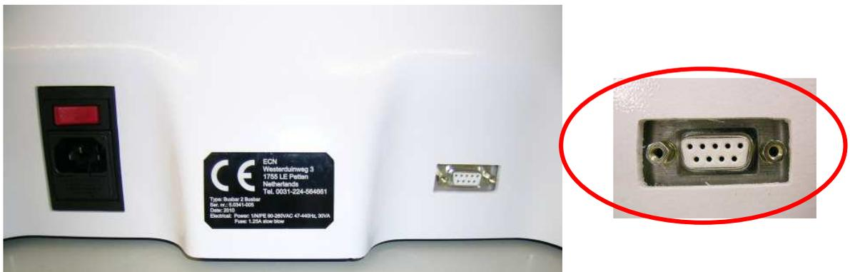
Figure 4.6 *Interface connection SunLab B2B*
